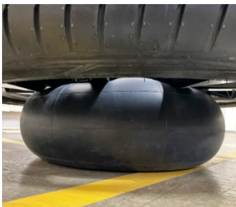
Fig. 3.3.1-12 Example of wheel support using a bike tire tube
