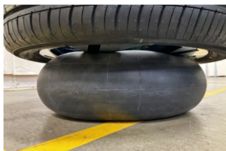
Fig. 2.2.2-1 Free-free boundary condition by rubber tube
