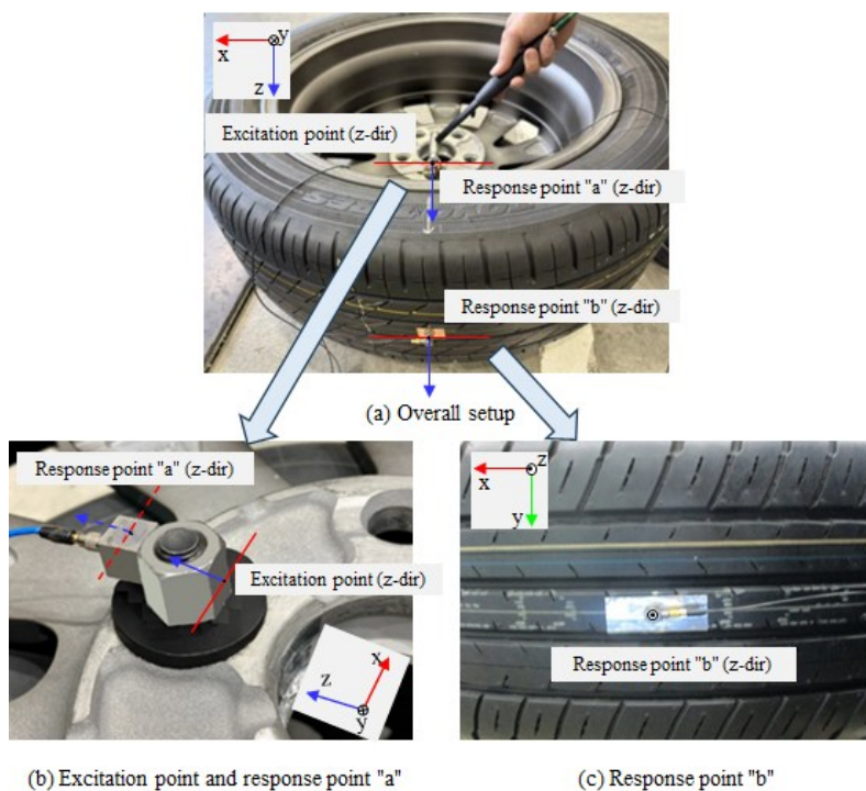
Fig. 2.2.2-2 Input and response points for force transmissibility measurement
